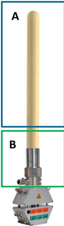
Area A is inside a furnace, and will radiate heat down to area B. The amount is different for each setup. Care must be taken not to overheat the region B. If the temperature is too low in the neck region B, consider using external means such as insulation or external heaters to increase the temperature in the neck.
