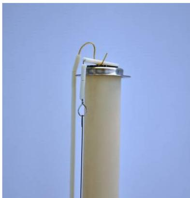
Lift the alumina spring load tube and the Au hook, and place the sample. Carefully lower the parts again so that the gold wire gently touches an area of no interest on the sample.
