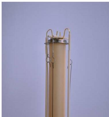
Mount the second set of alumina spring load assembly and upper electrode contact the same way as the first one. Now, lift up slightly the alumina spring load tubes and move the Au "hooks" to two selected electrodes.
