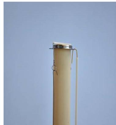
Place the top of the spring load assembly over the middle of the Pt cup and connect the two long springs. The end of the spring hook should point towards the sample support tube. Hook the springs to the pedestal rim.
