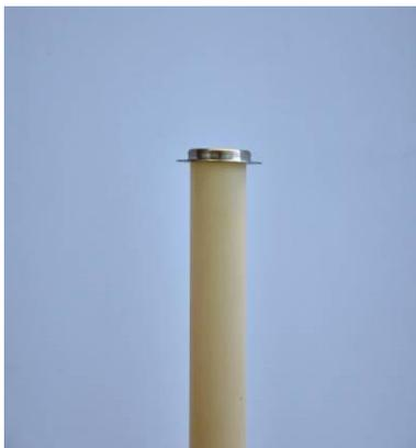
Mount the 16 mmØ sample support tube on the base unit. Place the Pt cup on top of the tube.
