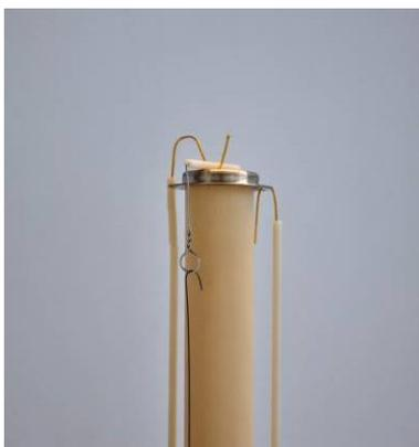
Connect the female contact of an Au electrode contact to one of the feedthrough connectors. Insert the upper, flat end so that it is held in place by the alumina spring load tube.
