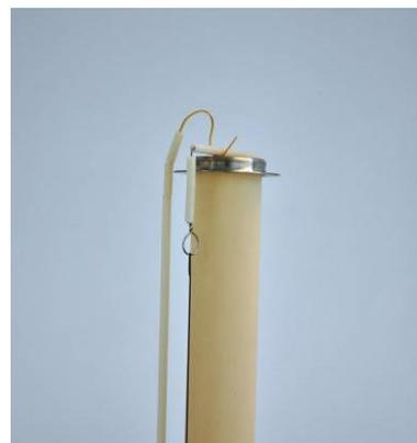
Au electrode contact: Connect the lower end to an appropriate feedthrough connector. Hook the upper, flat end so that it is held in place by the alumina spring load tube.
