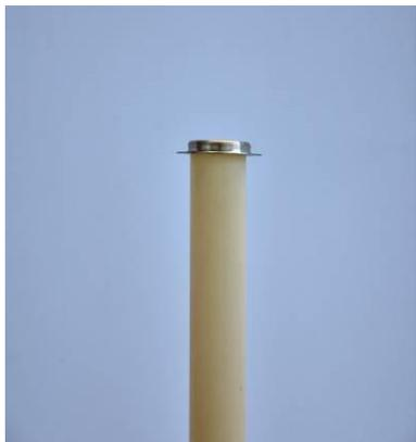
Mount the 16 mmØ sample support tube. Place the Pt cup on top of the tube.
