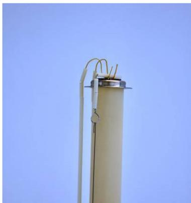
Mount the second upper electrode contact the same way as the first one. Now, lift up slightly the alumina spring load tube and move the Au hooks to two selected electrodes.
