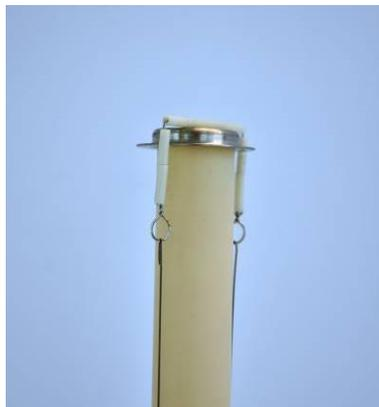
Spring load: Place the top part of the spring load assembly on the middle part of the Pt cup and connect the two long springs. The end of the spring hook should face towards the sample support tube.
