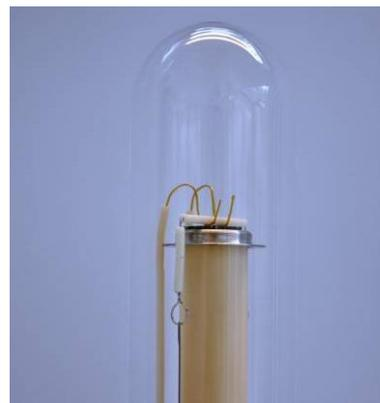
Lower the enclosing tube gently so that the setup is not touched. Secure the enclosing tube with O-ring and outer flange.
