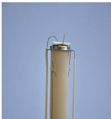
Lift the alumina spring load tube and the Au hook, and place the sample. Carefully lower the parts again so that the gold wire gently touches the selected sample electrode on top of the film.
