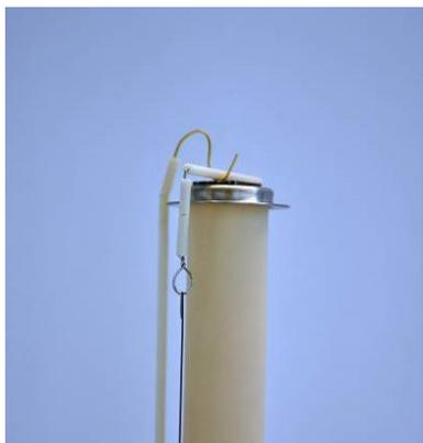
Lift the alumina spring load tube and the Au hook, and carefully place the sample. Carefully lower the parts again so that the gold wire gently touches an area of no interest on the sample.
