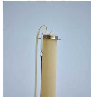
Au electrode contact: Connect the lower end to one of the feedthrough connectors. Hook the upper flat end so that it is held in place by the alumina spring load tube.
