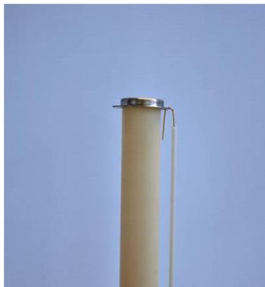
Hook the end of the lower Au electrode contact through one of the holes in the Pt cup, and connect its female contact to one of the feedthrough connectors.
